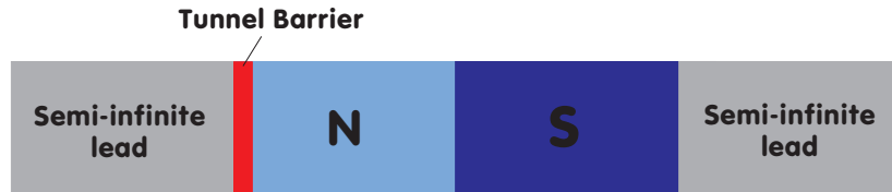
Figure 2. A N-S system with a tunnel barrier present. Such a system will have Andreev bound states present in the region between the interface and the tunnel barrier.
